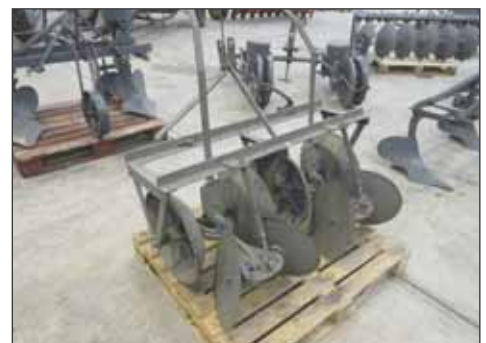
358 Geo. Henderson Ltd, Kelso mounted two row scarifier/bedformer
