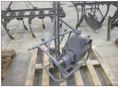
328 Ferguson Irrigation Pump, a simple centrifugal Beresford Model KG300 pump and primarily for the export market to service small mechanised farms
