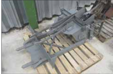
307 Ferguson Winch mounted pto driven with land anchor, manufactured by Hesford, Ormskirk, W-UE-20
