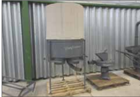
311 Ferguson Electromatic Hammer Mill fitted with multi-sack attachment and Scotmec electric power grinder. This is reported to be the only Ferguson implement not attached to a tractor or taking power from it
