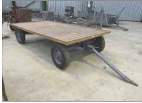
400 Ferguson 3ton 4wheel flat bed wagon. Only offered in North America W-JO-22
