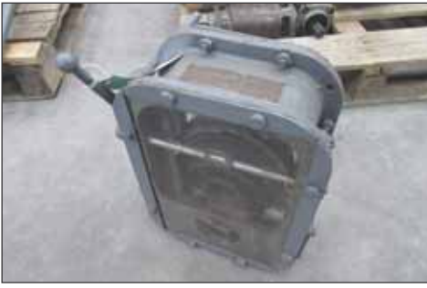
112 Ferguson Type A-TE-118 epicyclic demonstration reduction gearbox
