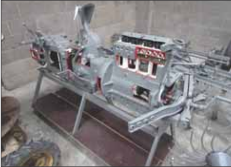
113 Ferguson TE-20 cut away demonstration tractor a fine sectioned exhibit with all the internal working parts exposed, operation by turning the starting handle. Created by J E Moffitt and a team of engineers and rebuilt with cut away sections, mounted to mobile trolley
