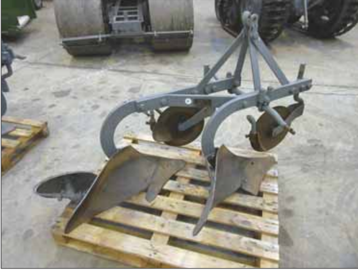
441 Ferguson Brown Type B10 mounted semi-digger 2furrow plough with discs and skimmers
