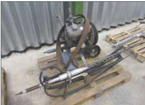
303 Ferguson Hydrovane 25CFM compressor commonly used with a hedgecutter or similar attachment
