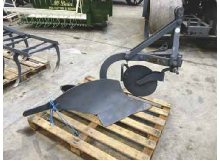
442 Ferguson Brown Type B10 Single furrow mounted plough with disc and skimmer (not attached)
