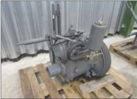
302 Ferguson Hydrovane 60CFM compressor used for heavy duty work such as road and concrete breaking, Sn.Z42075
