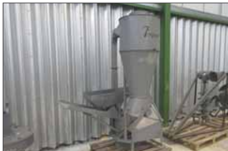
312 Ferguson Hammer Mill mounted with drive taken from a belt and pulley, H-LE-A20 Sn.1673
