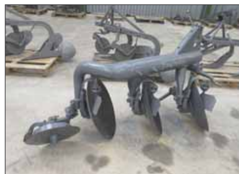
343 Ferguson 3furrow mounted disc plough with skimmers, rear wheel and support stand, P-AO-21 Sn.20304
