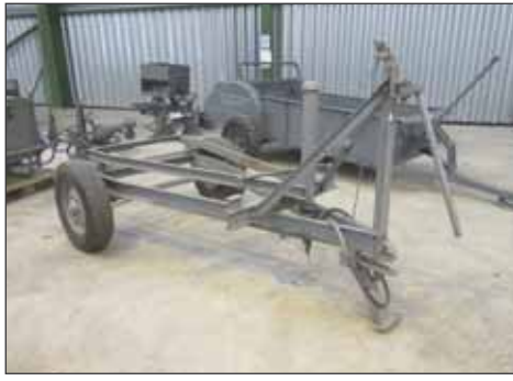
401 Ferguson (USA) trailer chassis with capacity of 4,000lbs. Ferguson's first trailer with rear wheel configuration, complete with weight transfer linkage and brakes. A most uncommon example built for the Ford 9N, JO Sn. 1818
